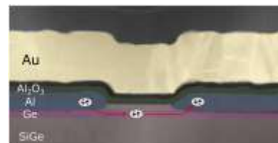
Fig.: Transmission Electron Micrograph of a Ge Josephson junction fabricated at the CEA clean room. (Courtesy of J. Labar, EK Budapest)
